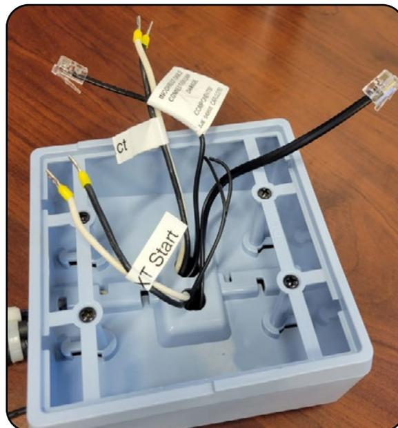
4. Connect all the Cables and wires to the correspond position in the T-Max.
