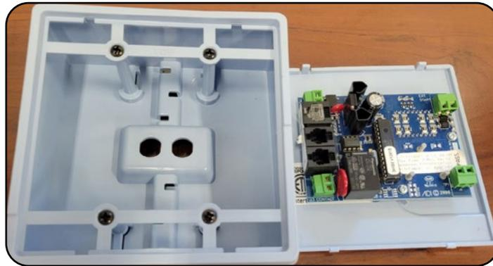
3. Trace cables on the back of the mount enclosure
